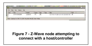
As seen above, the node also sends the data associated with its last known host. Although encryption is in place, it's possible (but ineffective due to timing constraints and the use of low power transmissions) to simply record the key set message and extract the key from there. Due to the used encryption, it is also possible and feasible to calculate all necessary keys from captured packets
