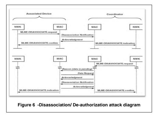
This key establishment scheme can be easily manipulated by the use of a De-Authorization attack. The node being detached is programmed to accept the network key established by the gateway.
