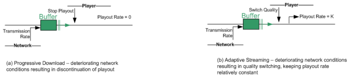
Figure 2: Progressive vs. Adaptive
