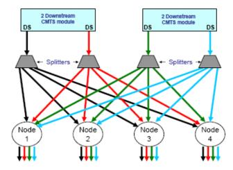
moving DOCSIS devices between interface to accomplish balanced subscriber counts and/or balanced utilization.
