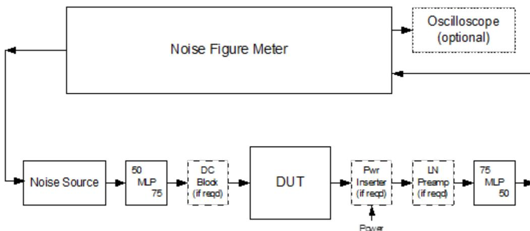
**Figure 2 - Measurement Setup**
