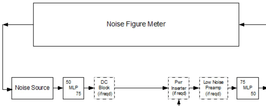
**Figure 1 - Calibration Setup**
