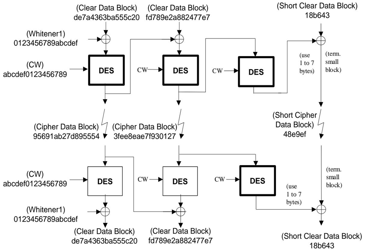
Figure 6 - Residual Termination Block Processing Example
