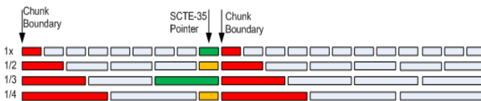
Figure 47 - Using AUs to Complete Chunk
