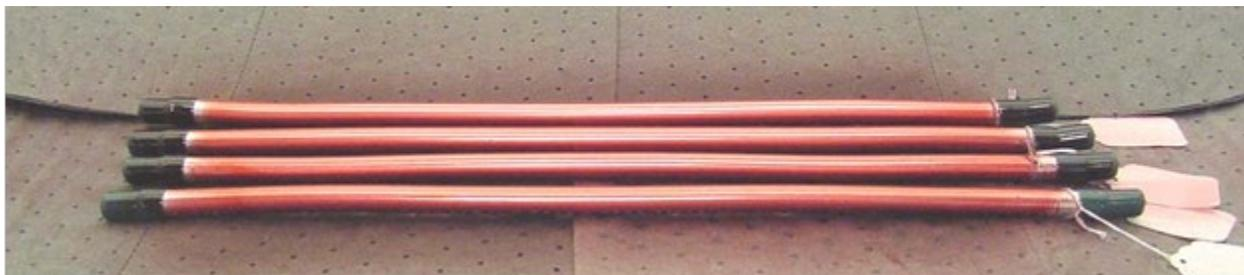
**Figure 2 - Samples with Penetrant Applied**
