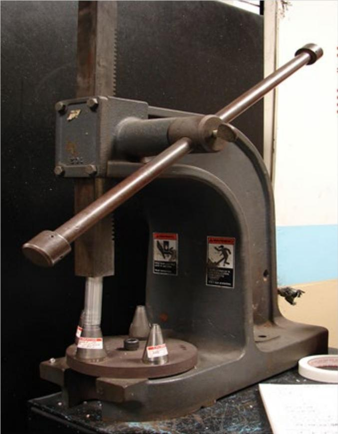
**Figure 6 - Mechanical Arbor Press**
