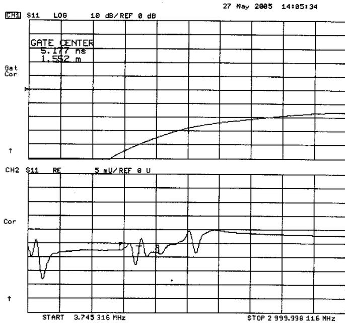
Figure 7 - Adjust Gate to Center DUT
