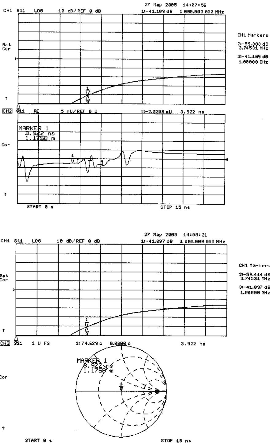
Figure 9 - Cable Impedance
