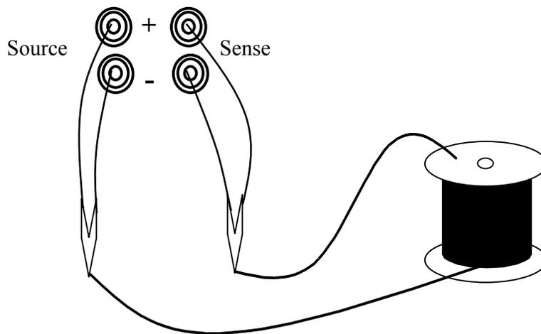
**Figure 1 - 4 Wire DC Resistance Measurement**
