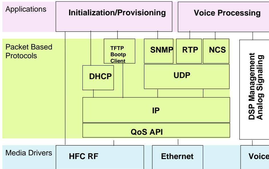
Figure 4. MTA Components
