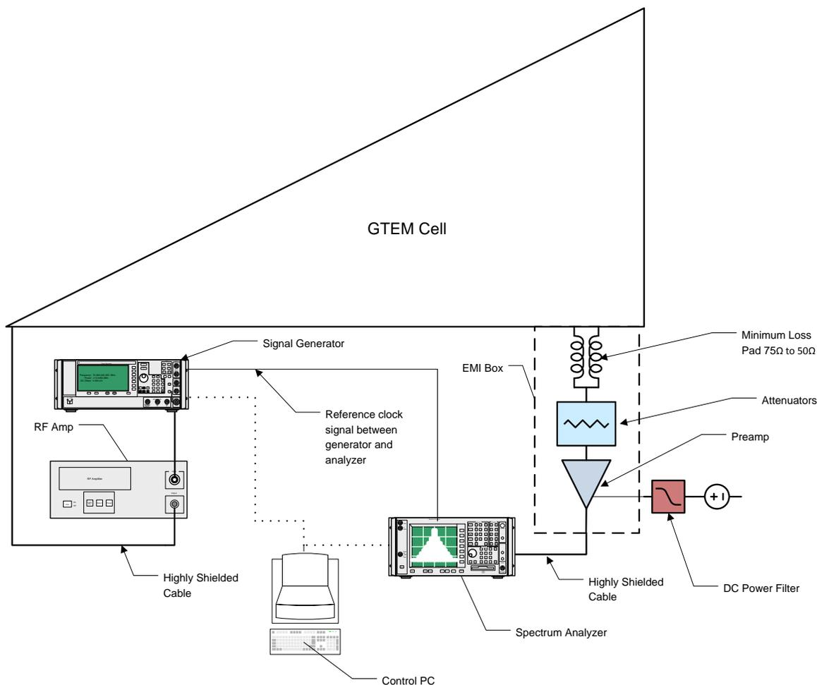
**Figure 3 – Test Configuration using Spectrum Analyzer**
