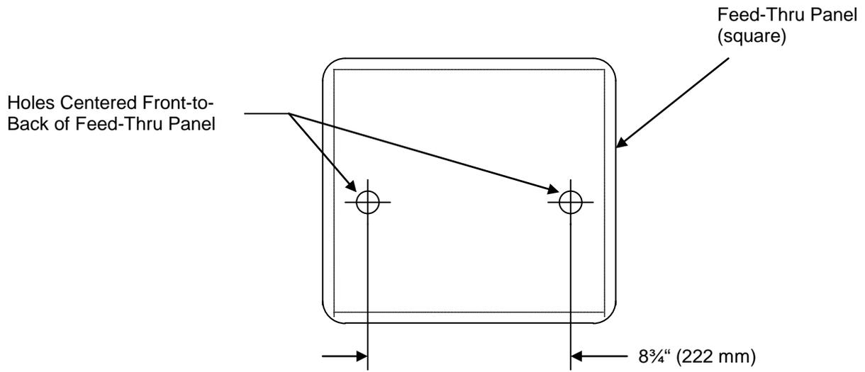
**Figure 10 – GTEM feed through panel with dimensions (Dimensions will vary with GTEM size)**
