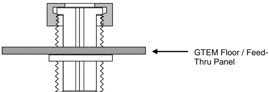
**Figure 12 – Typical feed-thru configurations**
