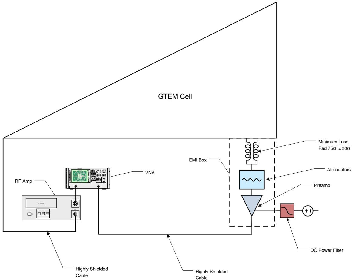
**Figure 2 – Test Configuration using Vector Network Analyzer**
