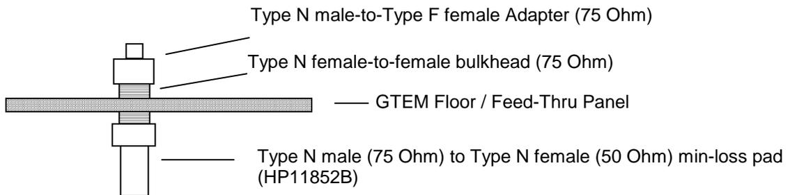
**Figure 11 – a typical feed-thru adapter setup used on the GTEM floor**
