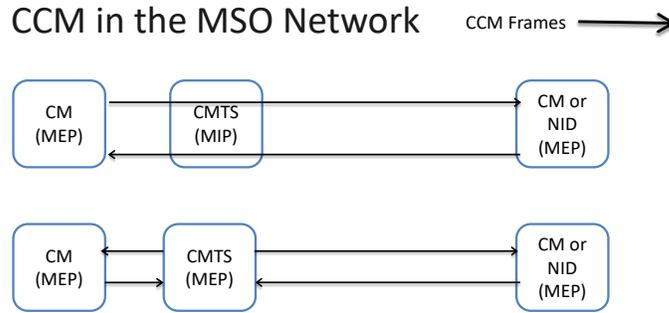
**Figure 8–2 - CCM in the MSO Network**
