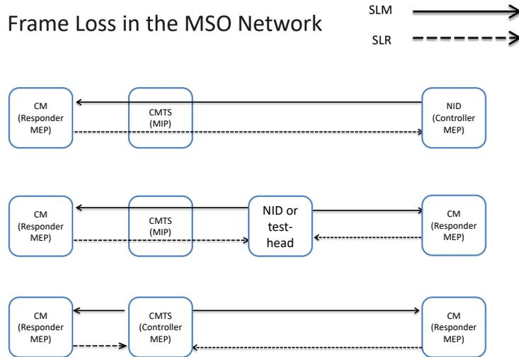
**Figure 8–6 - Frame Loss Functionality in the MSO Network**
