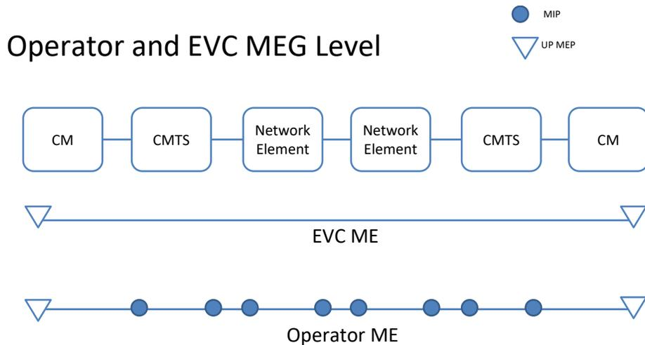
**Figure 8–1 - Operator and EVC MEG Level**
