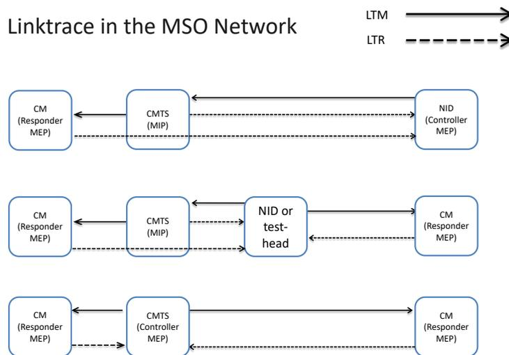
**Figure 8–4 - Linktrace functionality in the MSO Network**
