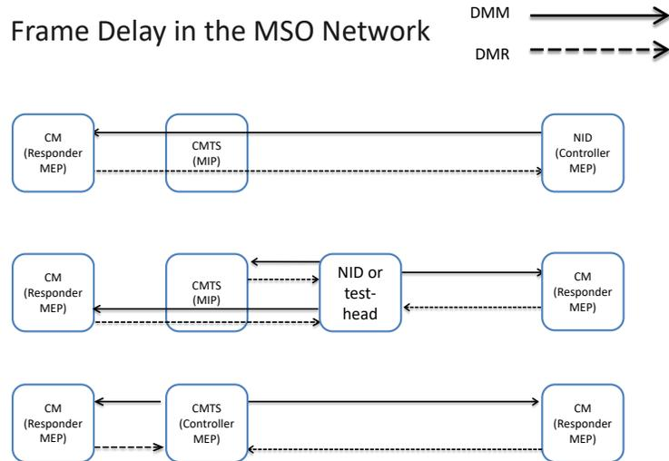
**Figure 8–5 - Frame Delay functionality in the MSO Network**
