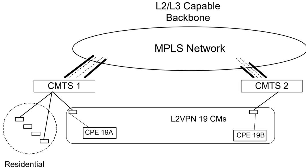
**Figure 5-2 - TLS over a MPLS Network**
