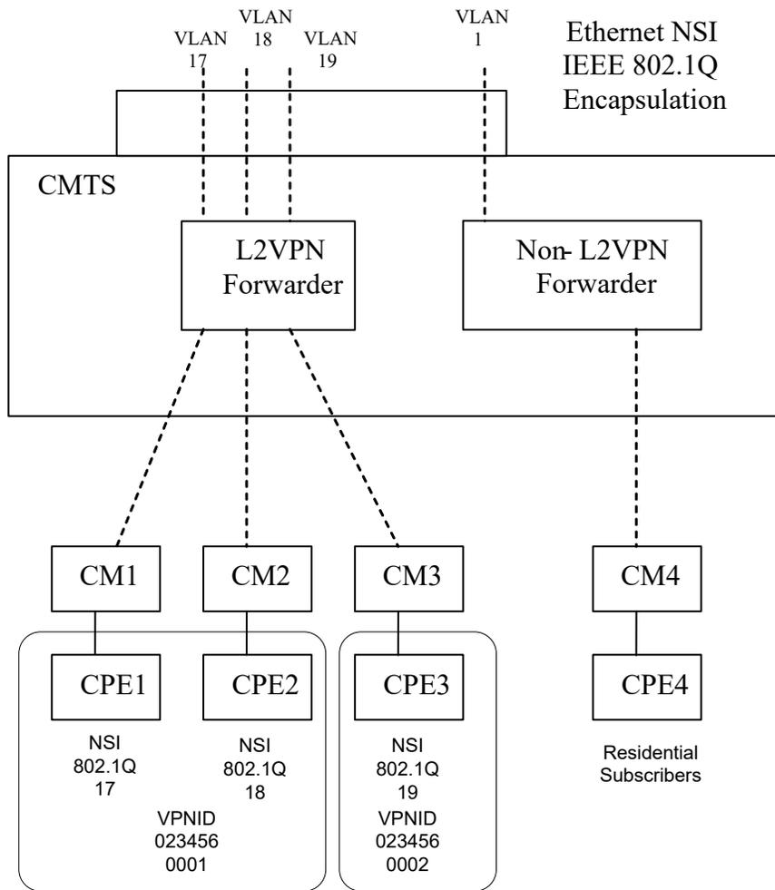
**Figure I-1 - Point-To-Point L2VPN Traffic Forwarding Example**
