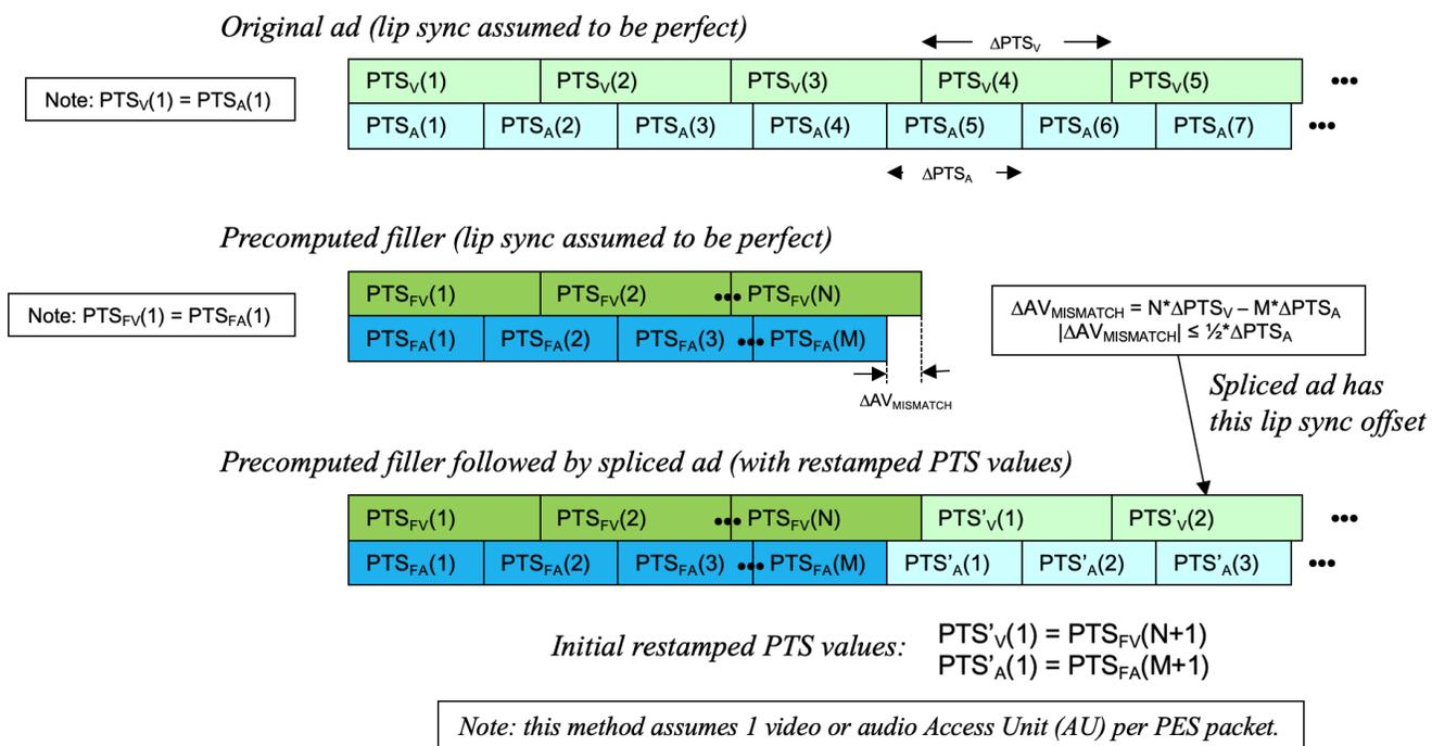
**Figure 10 Illustration of A/V presentation time mismatch introduced by splicing a perfectly synchronized ad after a perfectly synchronized Filler.**
