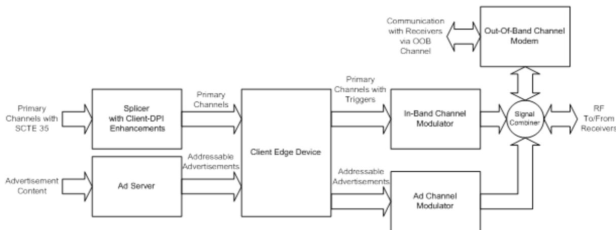
**Figure 5 - Example Level 0 Head-End Configuration #2**
