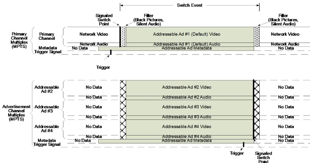
Figure 2 - Example Level 0 Transport Multiplex
