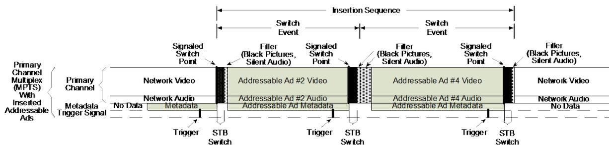
**Figure 3 - Back to Back Level 0 Addressable Insertions**
