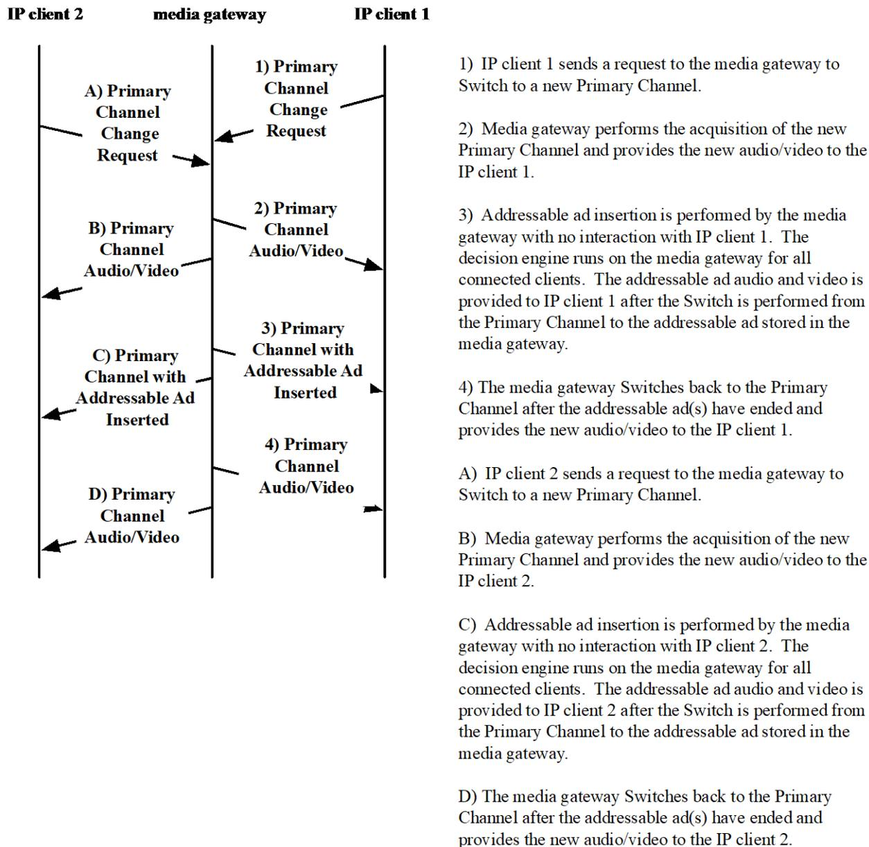
**Figure 1 – Media Gateway IP Client Communications**
