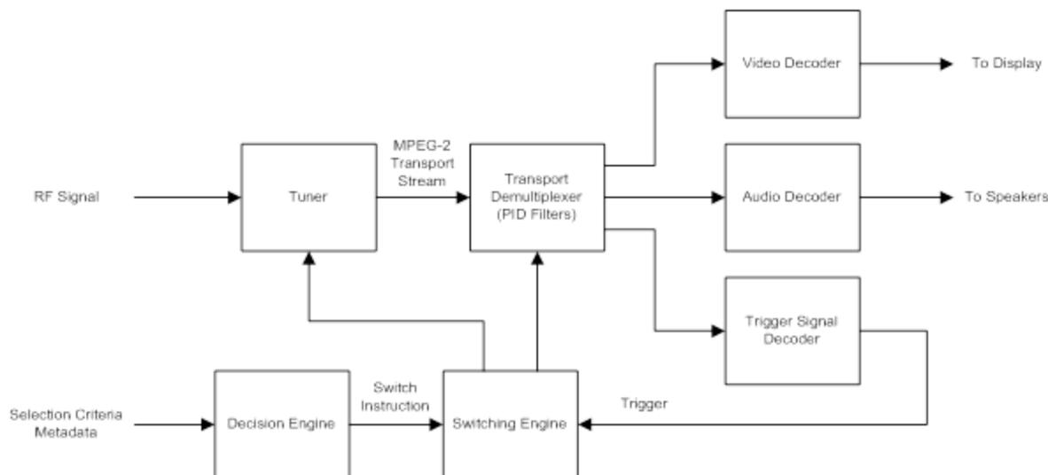
**Figure 6 - Example Level 0 Set-Top Decoder Architecture**
