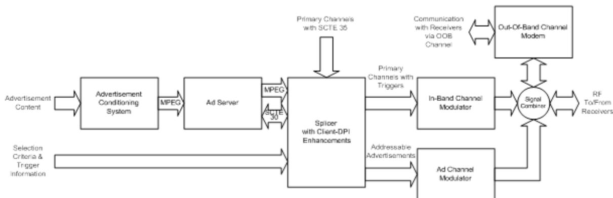
**Figure 4 - Example Level 0 Head-End Configuration #1**
