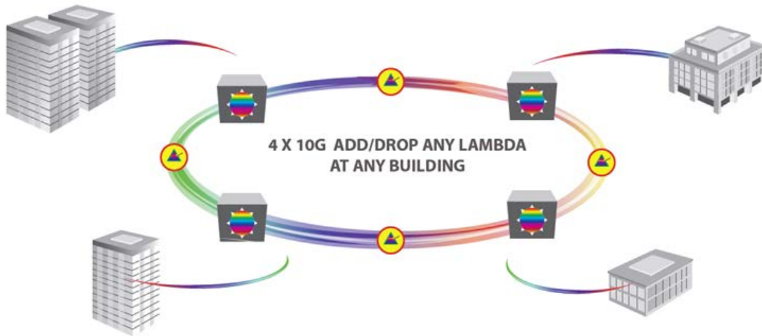
Figure 3 – Four Node WDM Ring with Four 10 Gbps Links Each
