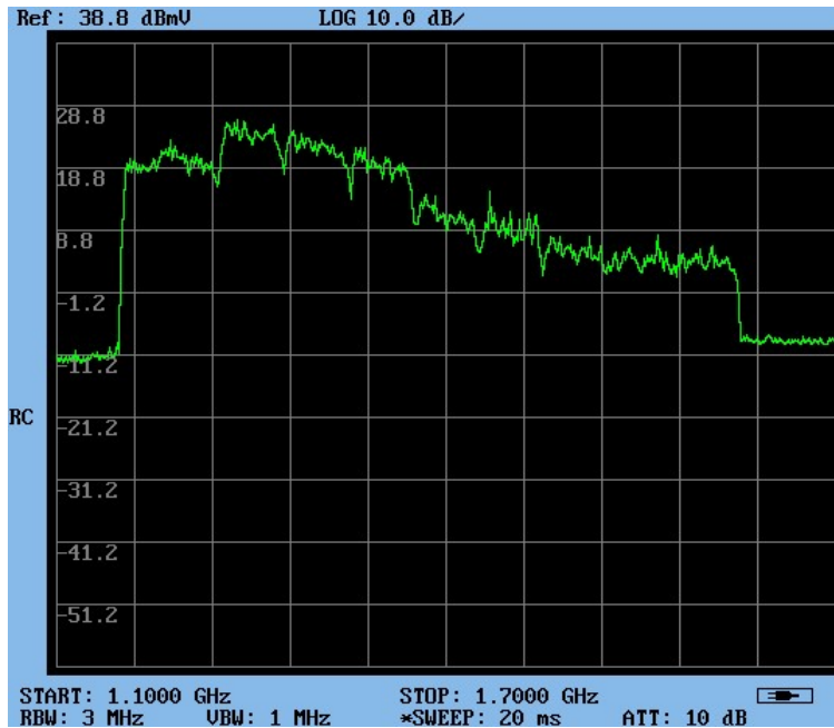
Figure 3 - OP2OP Isolation Of MoCA Exd OFDM Beacon Signals From D1 Thru D10
