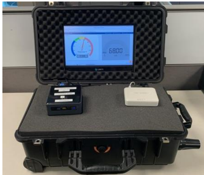
Figure 22 - LoRaWAN In a Box
