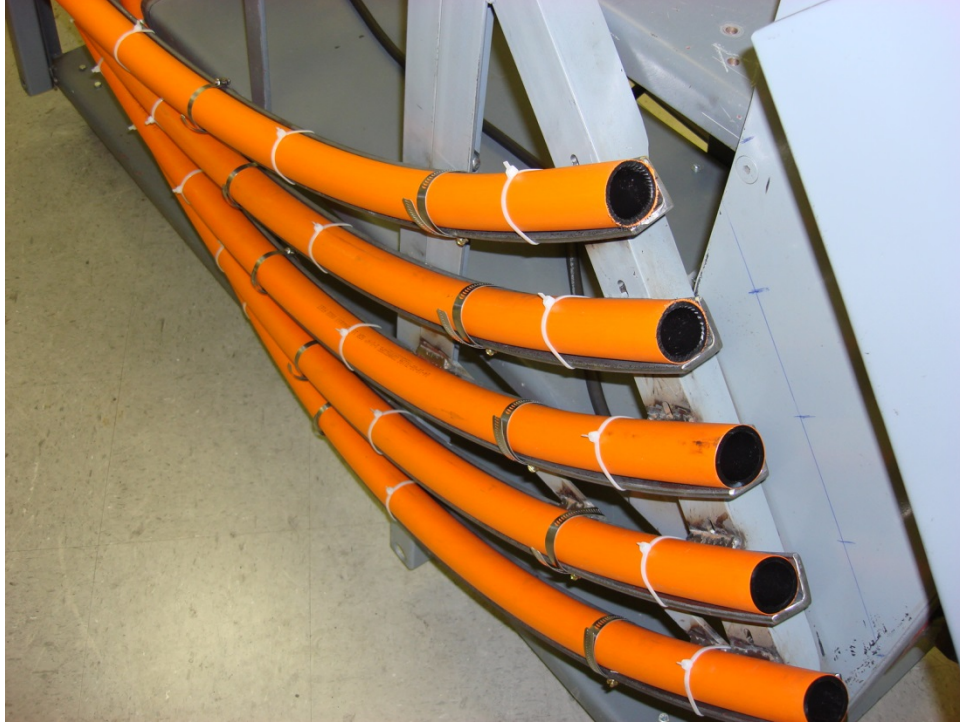
Figure 2 - Test Method A – multiple sample conditioner
