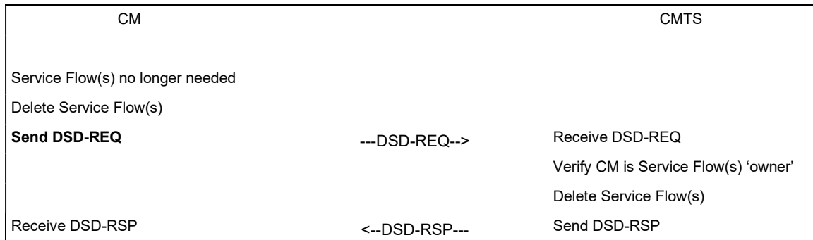
Figure 11–51 Dynamic Service Deletion Initiated from CM
