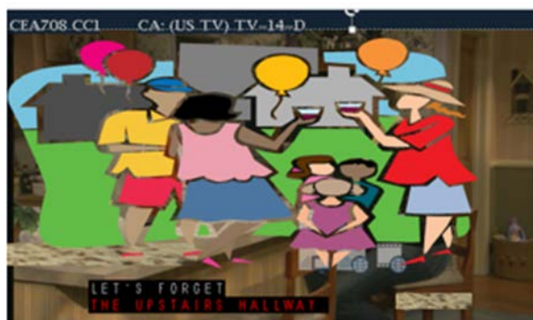
Figure 3 - The black text that was hidden in the black background is now shown in red using a Tektronix waveform monitor allowing the operator to quickly fix the problem.
