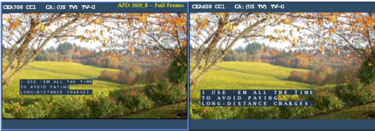
Figure 1 - This shows how a waveform monitor can be used to confirm the presence of 708 and 608 captions on the same DTV signal.
