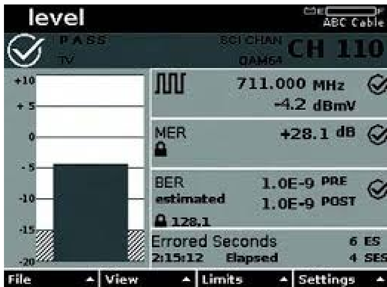
Figure 4. Digital channel power measurement using a cable TV signal level meter. Courtesy of JDSU (now Viavi Solutions, Inc.).
